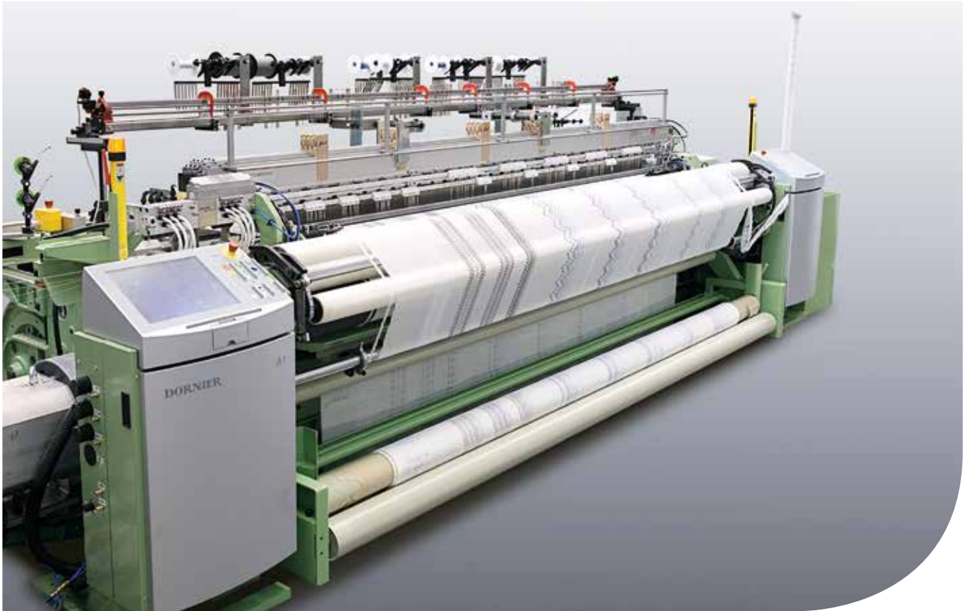
DORNIER A1 air-jet weaving machine with embroidery unit
